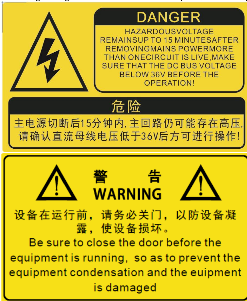
Figure 13: Warning Sticker Message on Inverter Front Door
